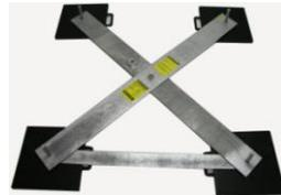
Slide the Top cross arm over diagonally opposite base weight pins.
