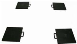
Lay the rubber coated base weights with suction cups facing downwards onto roof surface approx 1m apart. Ensure that the closest distance to any edge is not less than 2.5m
